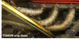
Keep heat inside pipes - increasing flow and lowering underhood temps
