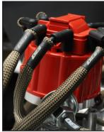
Protection for spark plug wires to prevent burning and cracking
