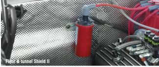
Block engine & header heat from getting into interiors
