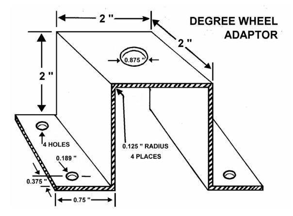
Material:Aluminum Flat Stock8" x 2" x .062" ST hardnessAlternate:Mild Steel Flat Stock8" x 2" x .040"
