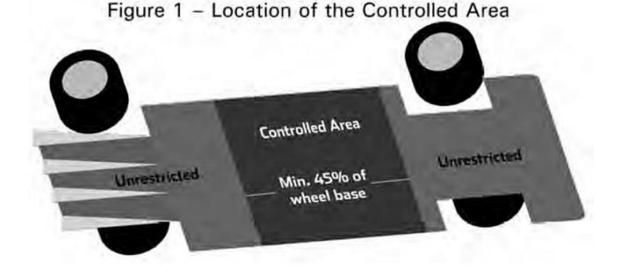
b. No aerodynamic devices (e.g. "skirts," body sides, etc.) may extend more than 1cm (0.394 inches) below this lower surface anywhere on the car to the rear of the front axle. Seat bucket or other protrusions shall not circumvent this rule.
