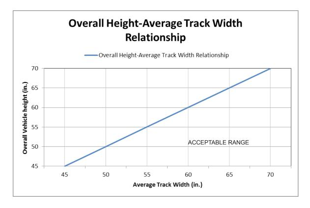
The measurements are to be taken from the ground to the tallest point of the vehicle for the Overall Vehicle Height and the normal track measurement as stated in Section 12.5 for the Average Track Width.
